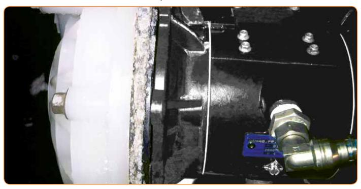
The aluminum materials in this air-operated double-diaphragm (AODD) pump had corroded at the diaphragm, leading to an extremely dangerous situation where workers were at risk of exposure.
