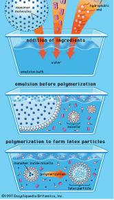
How Latex Is Produced By Emulsion Polymerization
