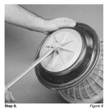
Using a 1" box wrench, adjustable wrench, or by rotating the diaphragm by hand, remove the diaphragm assembly.
