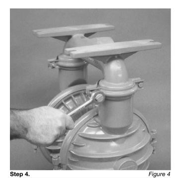
Remove the two small clamp bands that fasten the intake manifold to the liquid chambers. (Figure 4)
