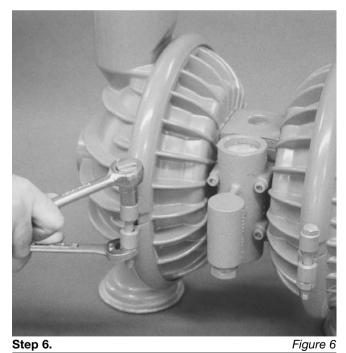
With % socket and 1% box wrench, remove one set of large clamp bands that attach liquid chamber to center section assembly. (*Figure 6*)
