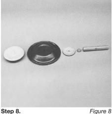
2) The outer piston, diaphragm, inner piston, and disc spring separate from the shaft which remains connected to the opposite side diaphragm assembly (Figure 8). Teflon®-fitted pumps come standard with back-up diaphragms (not shown).
