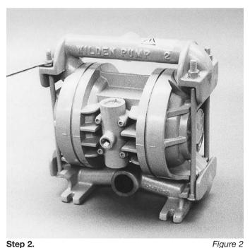
Utilizing the  $\frac{9}{6}$ " box wrench, start by removing the four long carriage bolts that secure the top and bottom manifolds to the center section. (*Figure 2*)
