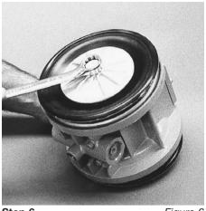
Step 6. Figure 6 With the <sup>3</sup>/<sub>4</sub>" box wrench or by rotating the diaphragm by hand, remove the diaphragm assembly. (Figure 6)
