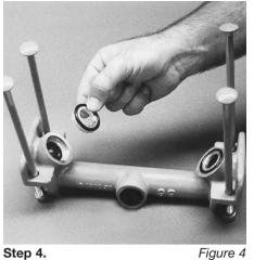
Remove the discharge valve balls, seats and o-rings from the discharge manifold and inspect for nicks, gouges, chemical attack or abrasive wear. Replace worn parts with genuine Wilden parts for reliable performance. Teflon<sup>®</sup> o-rings should be replaced when reassembled. (Figure 4)
