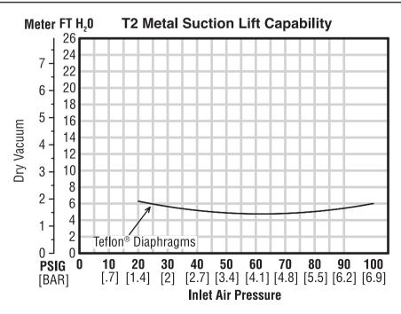
Suction lift curves are calibrated for pumps operating at 305 m (1,000') above sea level. This chart is meant to be a guide only. There are many variables which can affect your pump's operating characteristics. The number of intake and discharge
