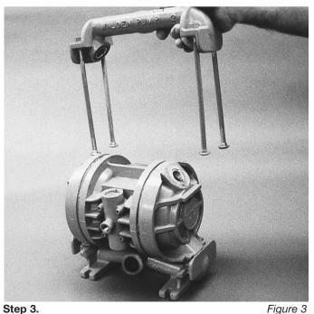
Remove the top manifold and lift the center section off the inlet manifold. (*Figure 3*)
