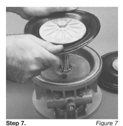
NOTE: Due to varying torque values, one of the following two situations may occur: 1) The outer piston, diaphragm and inner piston remain attached to the shaft and the entire assembly can be removed from the center section (Figure 7).
