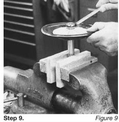
To remove the diaphragm assembly from the shaft, secure shaft with soft jaws (a vise fitted with plywood or other suitable material) to ensure shaft is not nicked, scratched, or gouged. Using an adjustable wrench, remove diaphragm assembly from shaft. Inspect all parts for wear and replace with genuine Wilden parts if necessary. (Figure 9)
