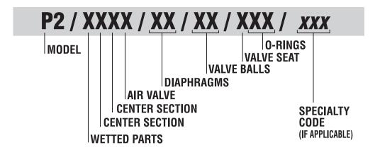
In the case where a center section is used instead of a center block and air chambers, the designation will be as follows: Polypropylene = PP
