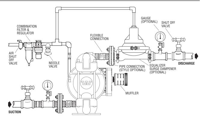
To stop the pump from operating in an emergency situation, simply close the shut off valve (user supplied) installed in the air supply line. A properly functioning valve will stop the air supply to the pump, therefore stopping output. This shut off valve should be located far enough away from the pumping equipment such that it can be reached safely in an emergency situation.
