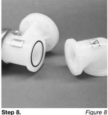
Normally inlet and discharge manifolds should not be disassembled during regular pump maintenance. Should this be necessary, completely remove clamp bands and inspect o-rings for nicks, cuts and chemical attack.
