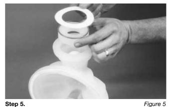
Carefully remove the protective covering from the back of the PTFE gasket attached to tape.
