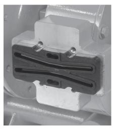
Be sure to note the orientation of the air valve gasket. (The flat side mates against the manifold and the grooved side faces the air valve.).
