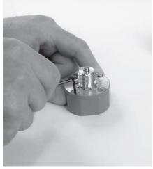
Using a 5/64" hex-head wrench, remove the four fasteners to disassemble the pressure relief valve.
