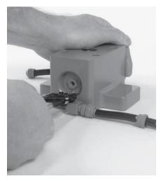
**Step 9**Using a pair of snap-ring pliers, remove the snap-ring from the bottom of the air valve body.
