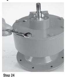
Using a 1/2" wrench, remove the fasteners that connect the power piston cylinder cover to the power cylinder body.
