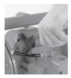
**Step 4**Using an adjustable wrench, remove each pressure relief valve.
