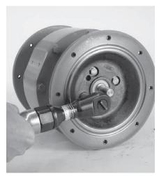
**Step 22**Using a 1/2" socket, remove the air chamber fasteners,
