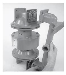
Hints & Tips – Due to the liquid chamber design, the pump can be positioned on one liquid chamber as shown; you can use the liquid chamber to assist with removal of the manifolds or opposite liquid chamber.
