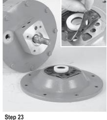
With the air chamber removed, note the orientation of the bushing and center section gasket.
