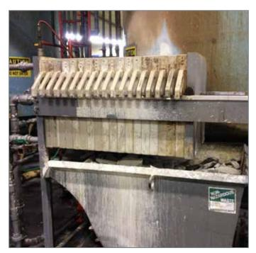
AMTROL's filter presses receive sludge containing water and metal particulate waste pumped by Wilden AODD pumps for separation into solid "sludge cakes" and water for safe, convenient disposal.
