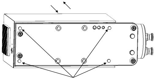
Loosen  $4x\ M6$  (wrench size 10) resp. fit for the assembly together with the washers
