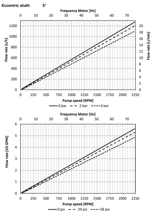
The flow rates showing at the charts above were ascertained with new diaphragms and new valves under standard conditions after the final assembly of the pump. Depending on the selected motor/frequency drive combination, the motor frequency and the resulting pump speed might differ.
