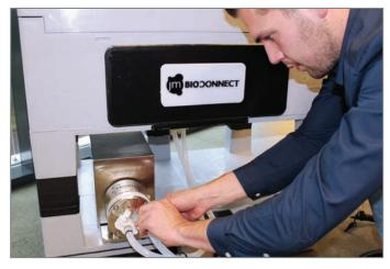
heart—which is eminently capable of pumping whole human blood, one of the most shear-sensitive products around—with its four pumping chambers and check valves keeping product flow constantly moving forward.
