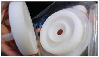
The QuattroMix<sup>™</sup> system has a very basic, easy-to-understand operating principle and includes a single-use mixing bag, a Quattroflow<sup>™</sup> pump and a 16-hole mixing plate that is built into the baq.
