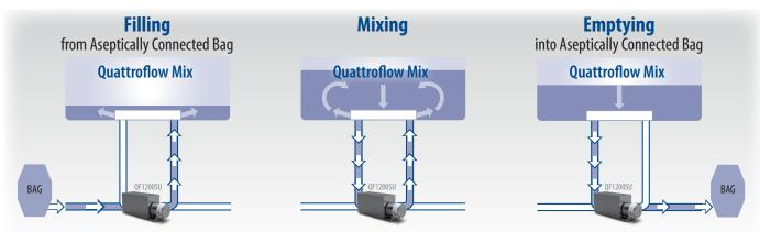
Another benefit of the QuattroMix" system is that filling, mixing, emptying and post-mixing filtration steps can all be accomplished by utilizing the same Quattroflow" pump.
