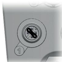
Fig. 21: Conductive rubber band in connection socket 1
