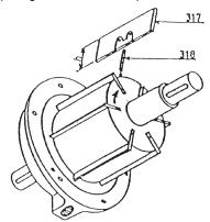
In case of abnormal wear, check the surface of the body and the faces of the end-plate. Refit the pushrods, making the holes in the rotor and the shaft coincide and making sure that the packing drive spigots are facing the notches in the rotor (see § REASSEMBLY).
