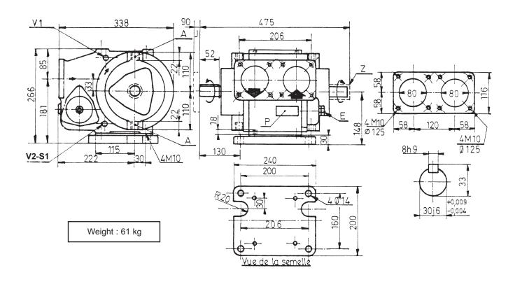
The pump has only one direction; depending on that of the power take-off, it will be driven by one end of the shaft or the other. In both cases, the position of the intake and discharge ports as well as that of the bypass remain fixed. It allows, nonetheless, rotation in the reverse direction at low speed and pressure to drain the lines.
