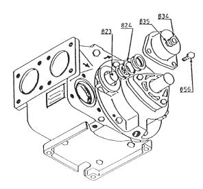
Make sure that the end-plate lies on the center line while it is being screwed down.
