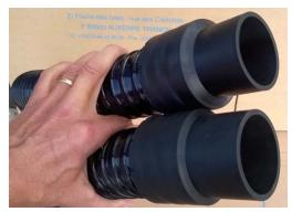
• To pass a heat-shrinkable sleeve on an end and to center it on the end of the hump. To retract gradually by means of a heat gun. Attention not to point the gun towards the hose not covered, risk of perforation.
