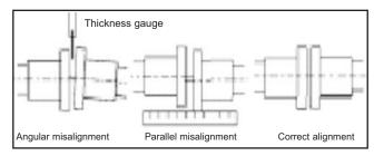
Figure 7- Coupling alignment
