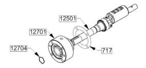
Fit the set bearing cage (12701 - 12703 - 12733 - 12627 and mechanical seal stationary seal face) on the shaft 12501.
