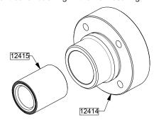
Orientate bushing chamfer on the outer side (see scheme above).
