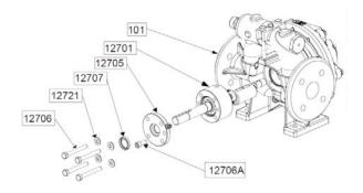
Fit the lip seal 12707, lip orientated outside in the bearing cover 12705.
