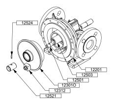
Lubricate the friction surfaces of the piston 12301O with a product compatible with the pumped liquid.
