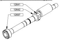
Check shaft 12501 surface condition. Rub it down with thin sand paper if there are scratches on seal rotating part O-ring place. In particular, it must be check that there are no scratches parallel to shaft axis.
