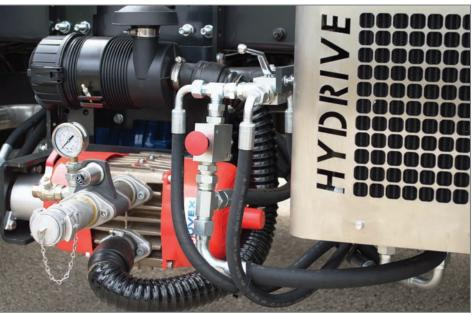
Mouvex® Enterprise Series Vane Compressors (left) and Hydrive® Hydraulic Coolers are ancillary equipment options that can be utilized when transport-truck loading and unloading activities need further optimization.
