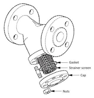
Put gasket on the cap. Put strainer screen on the cap and place assembly in the body and screw the nuts.
