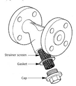
Put gasket on the cap. Put strainer screen on the cap and place assembly in the body and screw.
