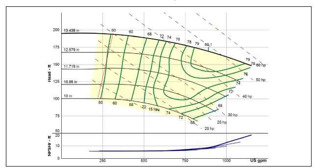
850 Series Model: 850FM/6X5-14T/4P PEl<sub>CL</sub> 0.96 Impeller Diameter: 13.438 in.
