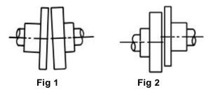
ANGULAR MISALIGNMENT as shown in Fig.1 should be corrected before eccentricity. Refer Fig.3. Use feeler gauge reading at 90° intervals, the amount of correction necessary can be easily determined to bring shaft axes in line.
