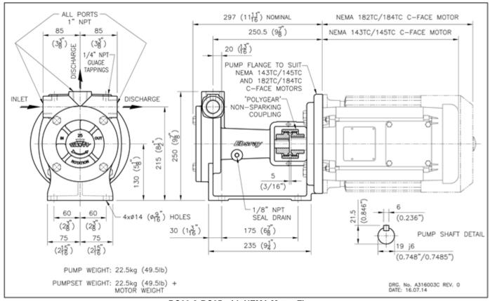
RC20 & RC25 with NEMA Motor Flange
