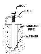
Figure 2. Foundation Anchor
