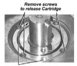
Insert screws to withdraw Cartridge
