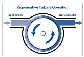
The design of a regenerative turbine pump is unique and works on a different principle than positive displacement pumps. This design, however, allows the pump to operate cavitation-free at speeds up to 3,800 rpm and at high differential pressures with low flow rates, which makes it ideal for use in Autogas-handling applications.
