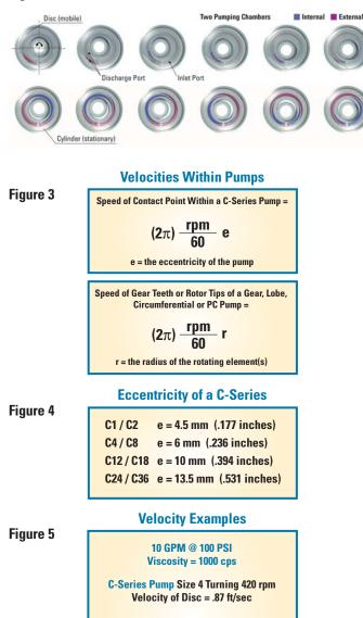
Typical Lobe Pump Size 18 Turning 340 rpm Velocity of Rotor = 3.15 ft/sec (based on a rotor diameter of 4.25 inches)
