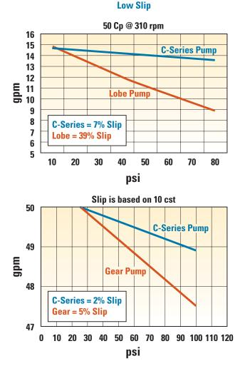
Blackmer Mouvex C-Series Eccentric Disc pumps are capable of handling viscosities up to 10,000 Cp, working pressures to 130 psi (9 Bar), capacities of 4 to 158 gpm (15.14-598.09 lpm), operating temperatures up to  $176^{\circ}$  F (80° C), and a particle size capability range of 1-3 mm. The C-Series is also very effective at handling suspended solids with mild abrasives.
