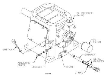
Figure 6 - Compressor Lubrication System
