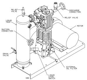
Figure 5 – Typical HD942 Compressor Package
