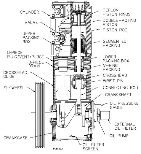
Figure 1 – Air-Cooled HD942B Compressor
