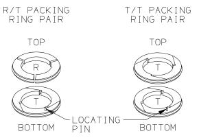
Figure 15 Packing Ring Detail
