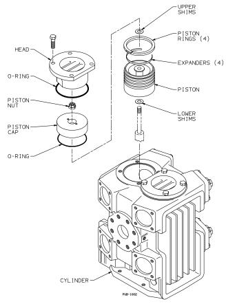
Figure 10 - Cylinder and Piston
