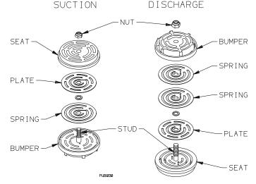
Figure 14 – Stainless Steel Valve Detail
