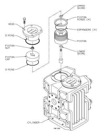
Figure 7 - Cylinder and Piston
