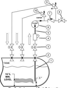
Fig. 5 – Underground Tank Schematic
