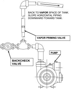
Fig. 6 – Vapor Priming Valve and Back Check Valve
