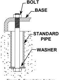
Figure 2. Foundation Anchor
