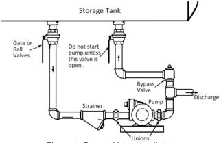
Figure 4. Bypass Valve Installation
