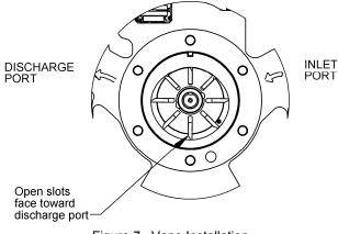
Figure 7. Vane Installation
