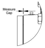
33. Remove bearing cap and install shims (26) with total thickness equal to measurement of gap between bearing cap and head. Reinstall bearing cap, and torque the capscrews (28) per Torque Table 1.
