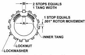
Figure 7 – Locknut Assembly
