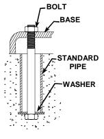
Figure 3 – Pipe Type Anchor Bolt
