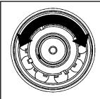
To check adjustment, grasp the nut and washer with fingers and rotate back and forth. If this cannot be done, one or both locknuts (24A) are too tight and should be alternately loosened one stop at a time (.001") (25 microns). Begin by loosening the locknut adjusted last. If used, tighten the locknut set screws (24C) securely.
