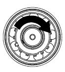
Tighten the opposite locknut (24A) by hand until it is snug against the bearing (24). Then, using a spanner wrench, tighten the nut the width of one lockwasher tang "B". Tighten just past the desired tang, then back off the nut to align the tang with the locknut slot. Secure the nut by bending the aligned lockwasher tang into the slot in the locknut. The pump should continue to turn freely when rotated by hand.
