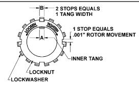
Back off the nut the width of one lockwasher tang "B". Secure the nut by bending the closest aligned lockwasher tang into the slot in the locknut. The pump should turn freely when rotated by hand.
