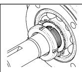
On both ends of the pump shaft, install a lockwasher (24B) with the tangs facing outward, followed by a locknut (24A) with the tapered end inward. Ensure the inner tang of the lockwasher is located in the slot in the shaft threads, bending it slightly, if necessary.
