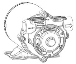
Figure 2 – Inlet and Discharge Port Locations
