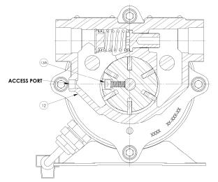
Figure 4: Rotor Capscrew Access
