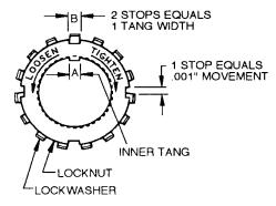
Figure 3 - Bearing Locknut Adjustment
