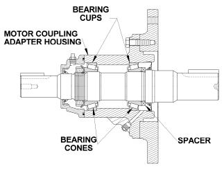
Figure 2 - Motor Coupling Adapter Assembly
