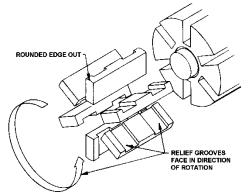
Figure 3 - Vane Installation
