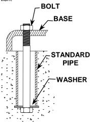
Figure 4 - Pipe Type Anchor Bolt
