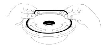
Figure 7 Head O-ring Installation
