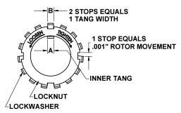
Figure 8- Locknut Assembly
