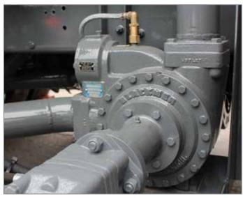
Only pumps that can reliably offer specific, steady, non-pulsing flow rates should be used on LPG delivery systems. For Robine Trucks, LGL Series Sliding Vane Pumps from Blackmer® meet these requirements.
