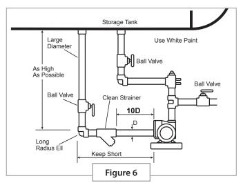
5. The nearest fitting or strainer should be a minimum of 10 pipe diameters from the pump inlet. Where possible, limit elbow connections to a maximum of 3 elbows. Use full port ¼ turn valves for component isolation. It is a good practice to install 3 full port ball valves, isolating the pump, bypass,
