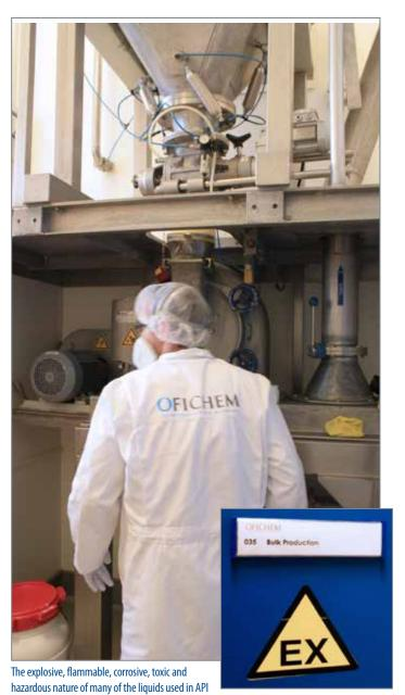
production require extreme handling precautions. Leak-free, ATEX-certified Almatec® AODD Pumps help ensure that the highest levels of safety are met.
