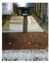
The pump's solidbody PE or PTFE block construction increases its strength and operational life cycle while eliminating many maintenance concerns. The pump's body and other components are CNC-machined rather than, as is the case with many competitive models, injection-molded.
