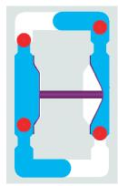
reached, it reverses automatically and the cycle is repeated in the opposite direction. In the second figure, liquid is drawn in by the left-hand diaphragm and displaced by the right-hand diaphragm. The liquid is displaced - and thus conveyed - by the compressed air. The diaphragms merely serve as barriers and are not pressurized, this is of critical importance for the service life of the diaphragms.
